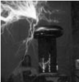
Overcoupling results in breakdown discharges that 'jump' down the secondary windings. Running the coil with lower coupling will reduce this, as will a larger, high-inductance primary. Notice in this photo that the breakdown occurred in the lower part of the secondary. When it jumps to the primary, it's known as D'Arsonval breakdown.
