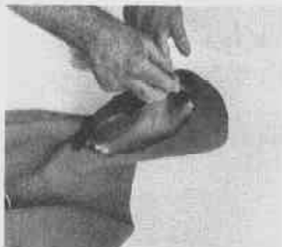
33. Apply cement to the outside surface of the entire seam joining the face-seal and hood. ALLOW THIS CEMENT TO BECOME TACKY—ALMOST DRY—BEFORE PROCEEDING.
