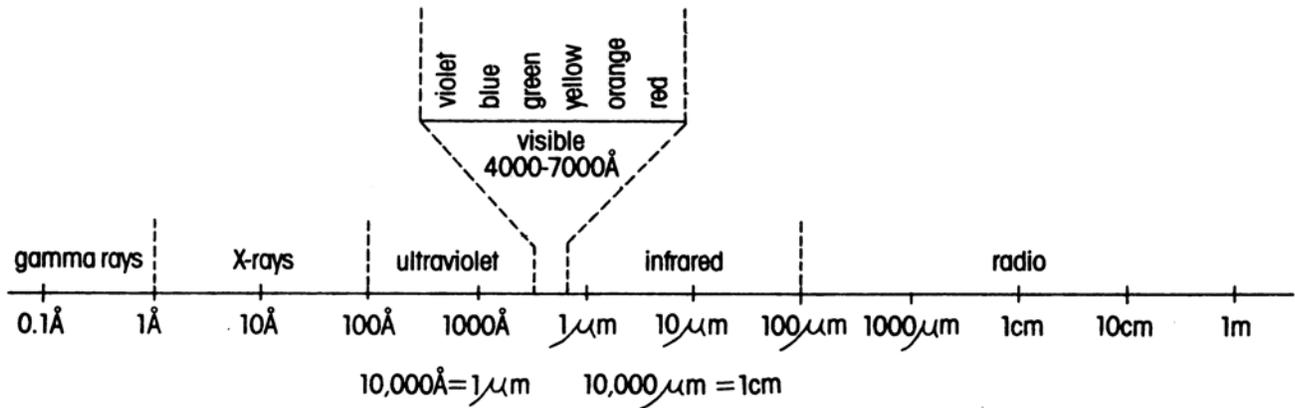
Schematic diagram of the electromagnetic spectrum, ranging from the shortest wavelengths (gamma rays) to the longest (radio waves). The wavelength of light is measured in Ångstroms (Å), micrometers (μm), centimeters (cm) and meters (m).
