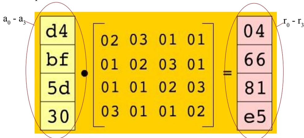
In this example, our  $a_0 - a_3$  is equals to d4 – 30 and  $r_0 - r_3$  is equals to 04 – e5. One thing to note in this is that it still follows the matrix multiplication rules: row x column. Currently the matrix size looks like this:
