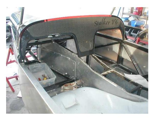
THE LEFT SIDE TUNNEL IS REMOVABLE TO ACCESS THE CLUTCH CYLINDER AND SPEEDOMETER SENSOR
