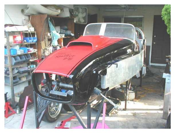
To keep developement costs low, the entire prototype, patterns and molds, as well as the jigs and fixtures to produce chassis and parts..were built in a 12' X 18' carport!!!!
