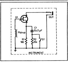
R1 (and an additional 5.1M resistor from the FET gate to ground) may be mounted in the cable jack.
