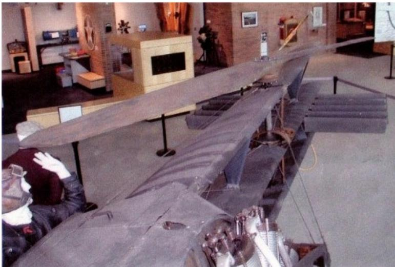
The front of the fuselage had the circular locating cuff for the engine cowl cut off, and the opening was covered over with plastic sheet. A hole was drilled in the middle to take the engine.
