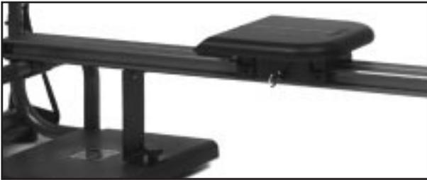
**Quick Release Bench:** The long portion of your bench attaches and releases from the seat portion very easily. To attach it, simply insert the half hinge on the end of the bench into the half hinge on the seat. For “standing” exercises, simply remove the bench by lifting up on the long portion and pulling away from seat.
