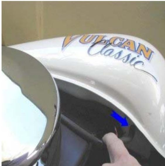
**d. [All Models]** Look/feel for the tank vent line on the right side of the tank towards the front; disconnect this line from the nipple on the fuel tank. Look/feel along this line for the tabs that secure it to the inside of the seam of the tank; free the line from these tabs and allow it to hang.
