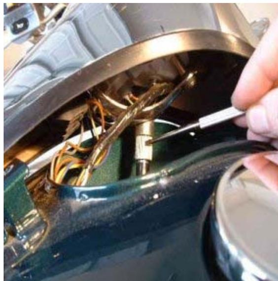
**1.** Unscrew the speedometer cable from the bottom of the speedometer.
