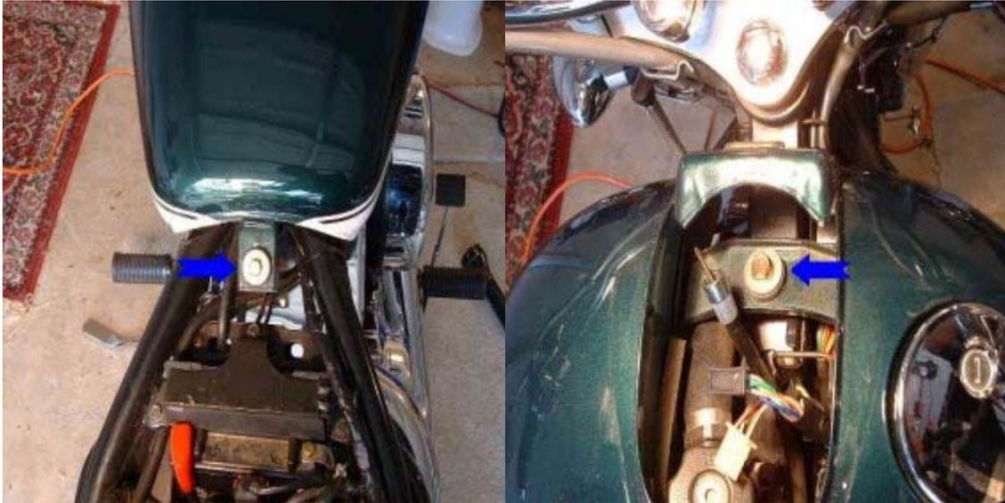
e. Remove the 12mm bolts at the rear and front of the tank. Lift the tank free, being careful not to tangle the crossbrace with the speedometer cable or instrument wiring.
