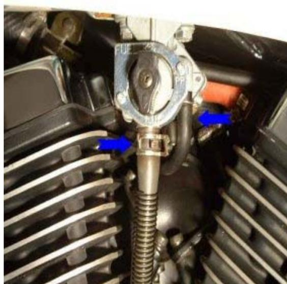
b. Ensure that the fuel petcock is in the **ON** or **RES** position; *not* in the **PRI** position! Disconnect the main fuel line (large hose) from the bottom of the petcock on the left side of the tank.
