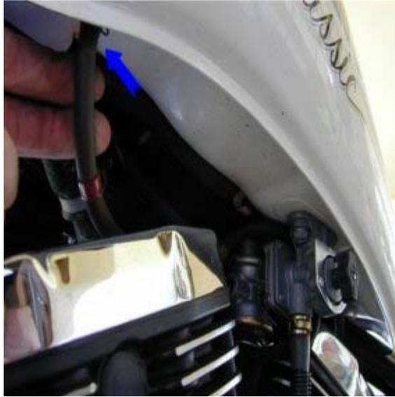
**d. [California Models]** Look/feel for the fuel vapor recovery line on the left side of the tank towards the front; disconnect this line from the nipple on the fuel tank. Look/feel along this line for the tabs that secure the line along the inside of the seam at the bottom of the tank; free the line from these tabs and allow it to hang. Repeat for fuel vapor recovery line on the right side of the tank, if present; if so, label this line to differentiate it from the tank vent line.
