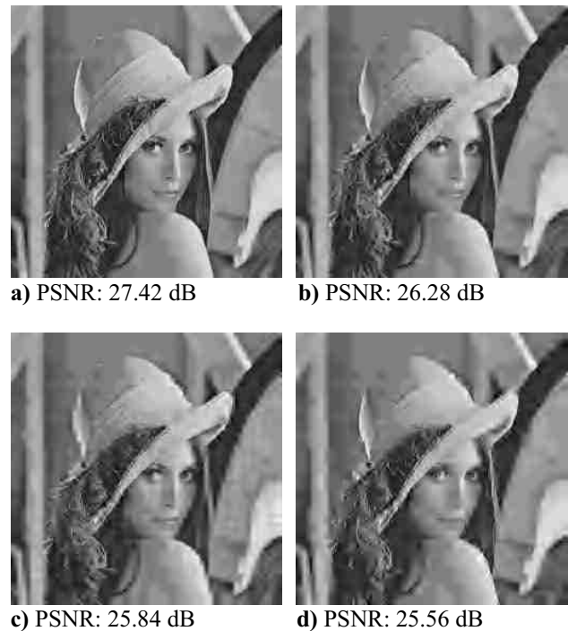
Figure 3: PSNR (dB) results for test image "Lenna" coded with Scheme 3 for Doppler spread a) 3 Km/hr, b) 40 Km/hr, c) 120 Km/hr and d) 300 Km/hr and with 2 turbo decoder iterations for E_p/N_0=5.5 dB
